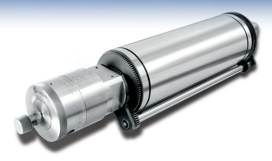
The AccuStrike<sup>™</sup> Anvil allows press operators to adjust blade clearance on press with extreme precision. Controls enable the operator to adjust bearers independently or together for unparalleled control over die strike on various liner thicknesses.
